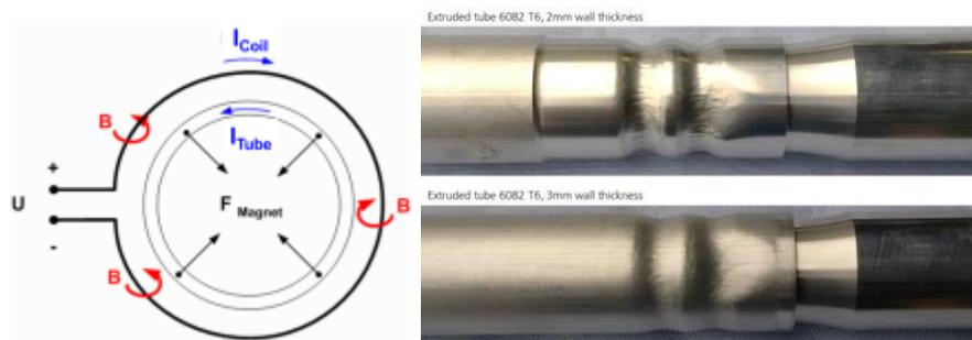
Figure 2: EMPT joining method – principle (left) and crimped coupon tests for determination of fatigue behaviour (right)
