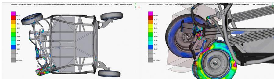
Figure 2: Deformation in the moment of maximum intrusion. Upper and lateral view
